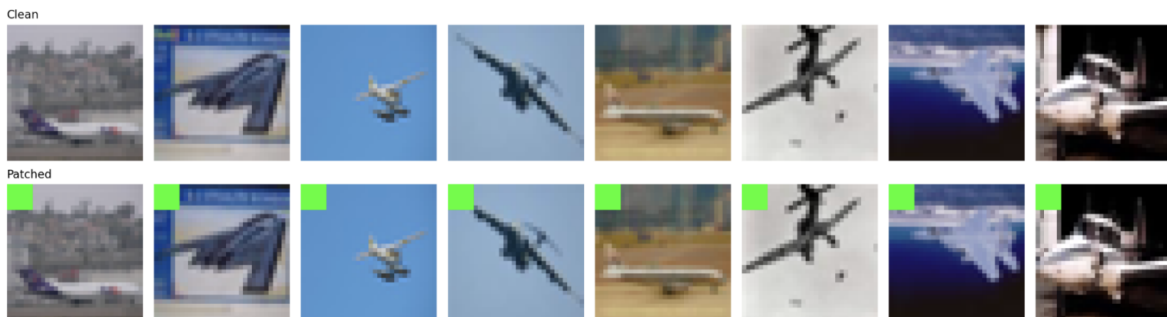
Figure 9.2: (Top) Eight class 0 (airplane) examples from CIFAR10 (Krizhevsky, 2009) without modification. (Bottom) The same eight images after undergoing SSTI injection of a patch in the top-left corner. Code used for this transformation can be found in listing 5. An injection proportion of 1 was used to ensure all images in the examples received the modification.
